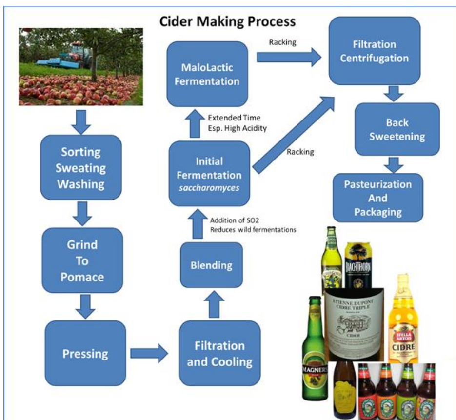
Scheme 1: A general outline of the cider making process for production of sweeter ciders. In drier cider production or bottle conditioned ciders the back-sweetening and pasteurization steps may be skipped.
