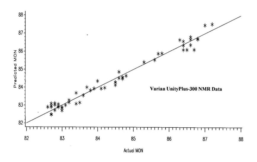
MON - D2699/D2700 Coefficients for NMR spectra - PLS w/ 10 factors (using centered NMR spectra) N=54 samples, SEP=0.24, Avg. error=0.20, Max. error=0.59, Bias=-0.007, R-sq=97.5
