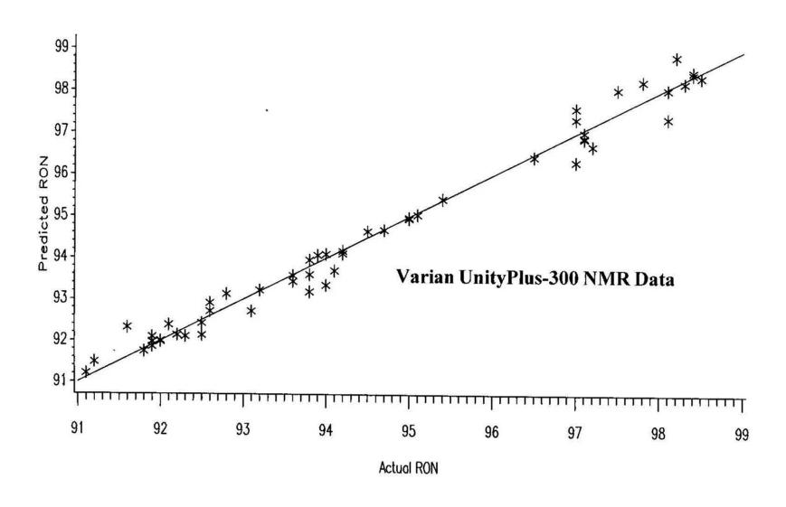
RON - D2699/D2700 Coefficients for NMR spectra - PLS w/ 14 factors (using centered NMR spectra) N=54 samples, SEP=0.31, Avg. error=0.22, Max. error=0.73, Bias=-0.005, R-sq=98.2
