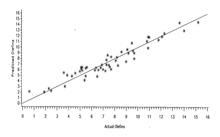
Olefins - GS-500 Coefficients for NMR spectra - PLS w/9 factors (using centered NMR spectra) N=54 samples, SEP=0.92, Avg. error=0.78, Max. error=1.88, Bias=+0.006, R-sq=91.2
