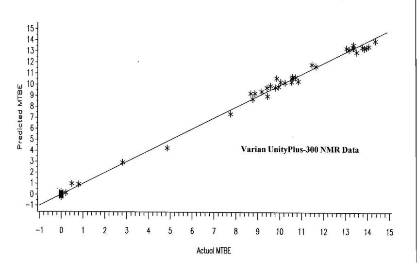
MTBE - GCOFID Coefficients for NMR spectra - PLS w/ 4 factors (using centered NMR spectra) N=54 samples, SEP=0.30, Avg. error=0.23, Max. error=0.79, Bias= $\pm$ 0.004, R-sq=99.7
