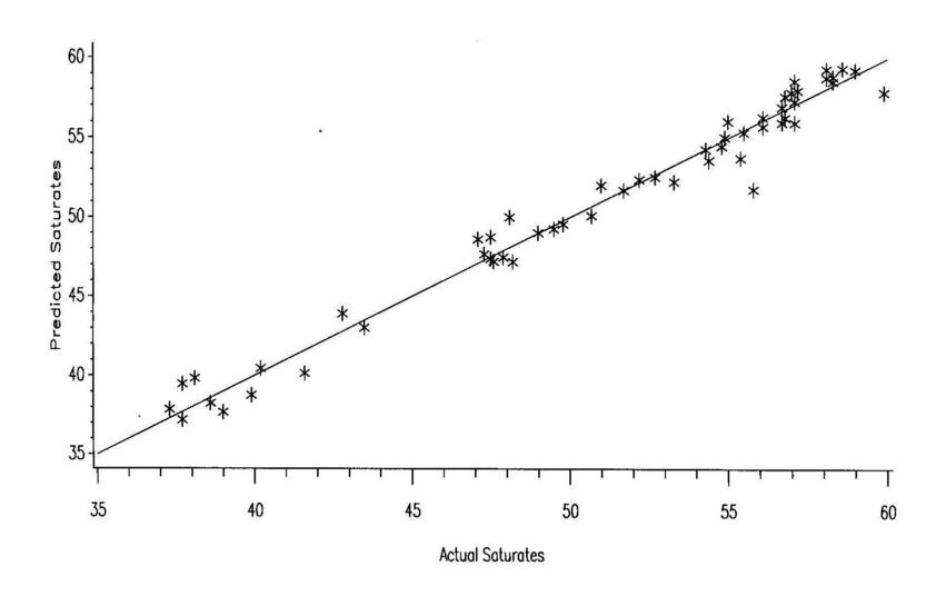
Saturates - GS-500 Coefficients for NMR spectra - PLS w/ 8 factors (using centered NMR spectra) N=54 samples, SEP=1.05, Avg. error=0.79, Max. error=4.04, Bias=+0.004, R-sq=97.6
