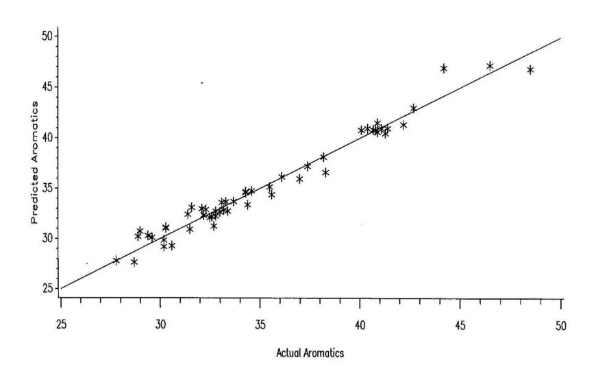
Aromatics - GS-500 Coefficients for NMR spectra - PLS w/ 8 factors (using centered NMR spectra) N=54 samples, SEP=0.86, Avg. error=0.67, Max. error=2.77, Bias=+0.007, R-sq=96.9
